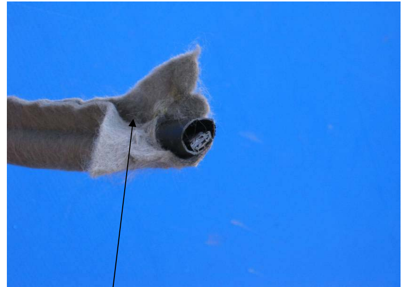
Geotextile conducts the water
